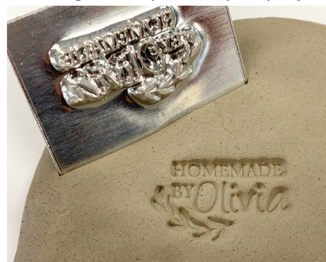
Magnesium mounted on aluminum block
