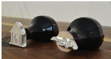
Magnesium dies mounted on wood handles
